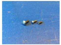
2. Shape the rivet head in electric drill using small files. Heads can be flat or more concave, with central hole or with dimple according to original shape of the rivet head seen on the vehicle.
