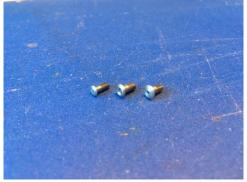
3. To make dark oxidized color of the steel rivet use Perma Blue liquid intended for repair of black surfaces of hand weapons. It is available in hardware shops or fishing and hunting shops.
